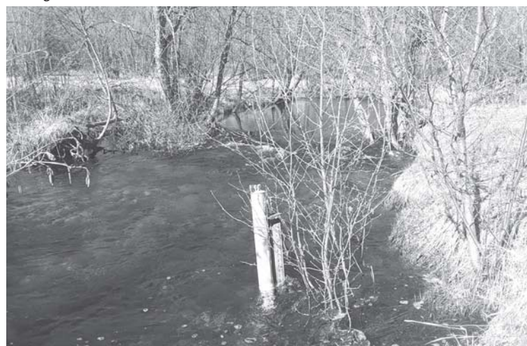
The Lazy Creek staff gauge and stilling well that houses a pressure transducer continuously measures stream level. Local lowland streams like Lazy Creek, Cow Creek, and Walker Creek typically see peak discharge in late April.
